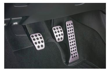
Answer key: the accelerator/gas pedal; brake; clutch
